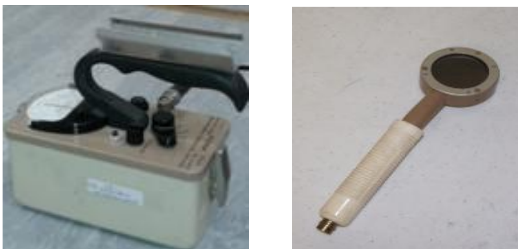
Figura. 4 Monitor Eberline E-120E Survey Meter e Sonda Thermo/Eberline Model HP-260 Pancake GM Detector
